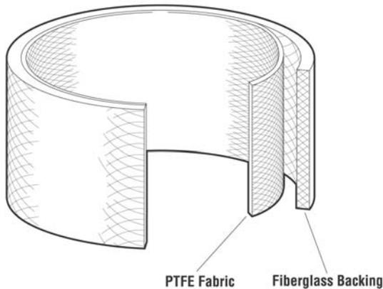
The structure of a properly designed self-lubricating bearing utilizes a high strength continuous fiberglass backing with a low friction, highly embeddable wear surface composed of high tenacity PTFE filaments.
