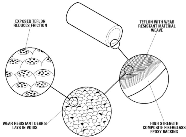
The above schematic represents a typical PolyLube™ self-lubricating composite bearing. The high strength composite fiberglass, epoxy resin backing with the PTFE wear-resistant liner combine to make an ideal product for the industrial equipment industry.
