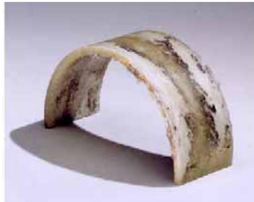
*In the case of this bearing, the edges of the bearing itself (seen in an almost white hue), show the misalignment generating a parabolic pressure curve that is in turn fatiguing the bearing backing.*
