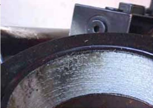
*PolyLube journal bearing liners employ a proprietary liner architecture that have engineered “pockets” that allow for the ingestion of contamination—regardless of the type of contamination in question. In the case of paint, the paint is quickly removed from the PTFE filaments and embed themselves into the pockets, allowing the bearing to continue functioning. This is a **unique feature** to the PolyLube Fiber and MRP family.*
